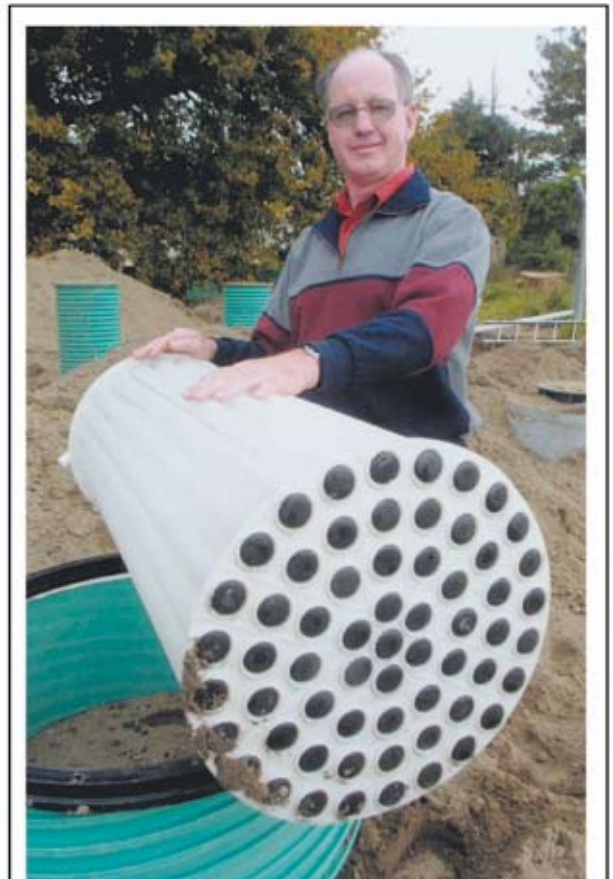
NEW-AGE SEWAGE: Environmental engineer Dave Miller with a bio-tube filter, part of the new sewage system at Hukarere Maori Girls College, Esk Valley. PHOTOGRAPH BY ANDREW LABRETT
